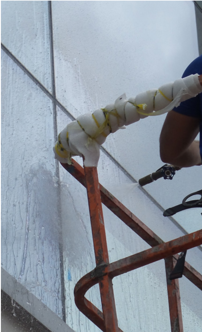
The spray nozzle is too close; AAMA 501.2 states the distance must be 305 plus or minus 25 mm (1 foot).
